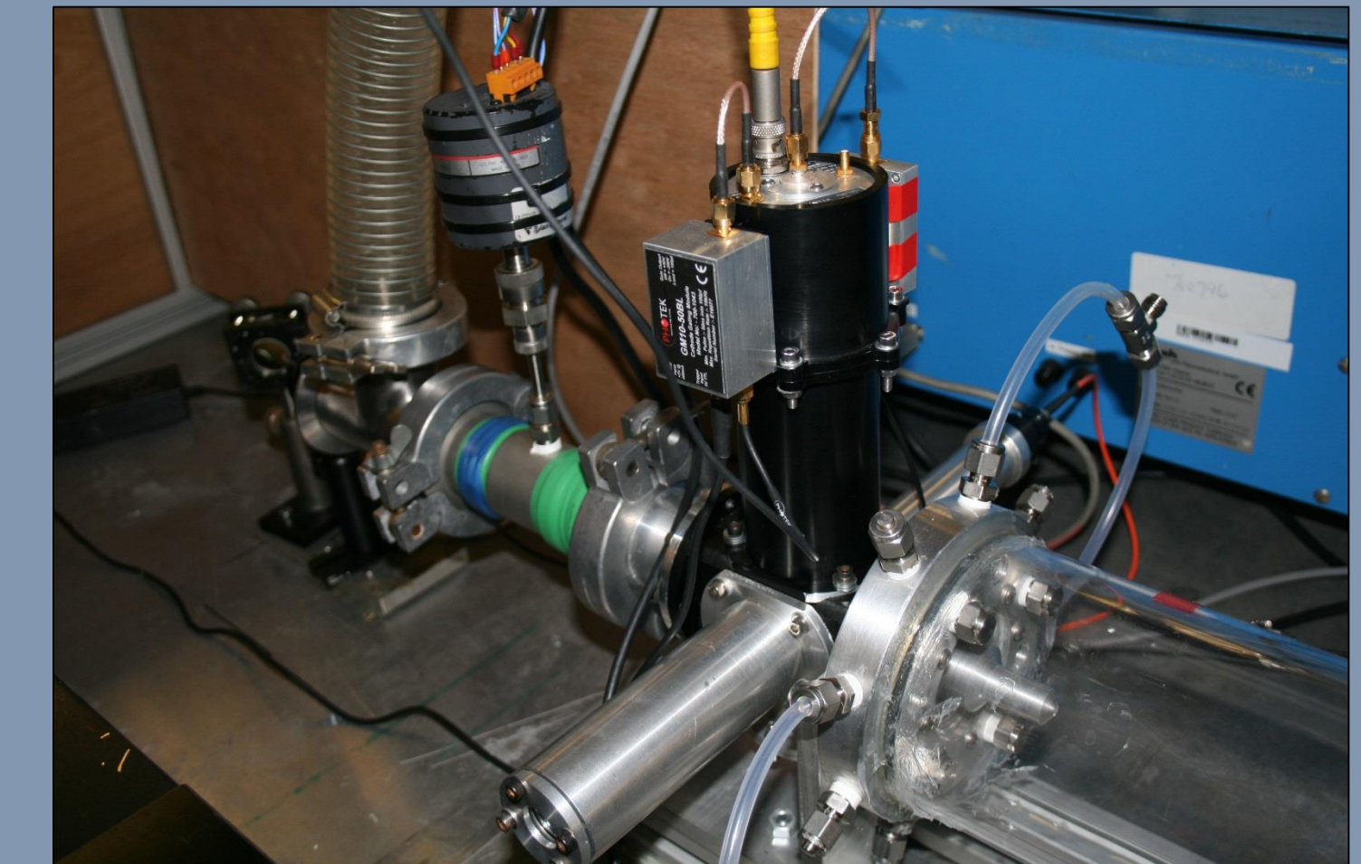
Figure 3. Image of the detection cell connected to the aerosol flow tube.
