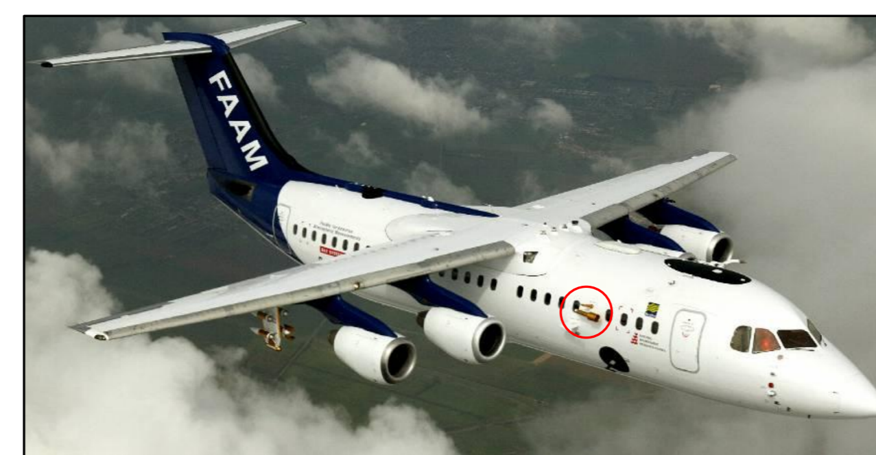
BAe-146 Research Aircraft, with HO x inlet circled in red
