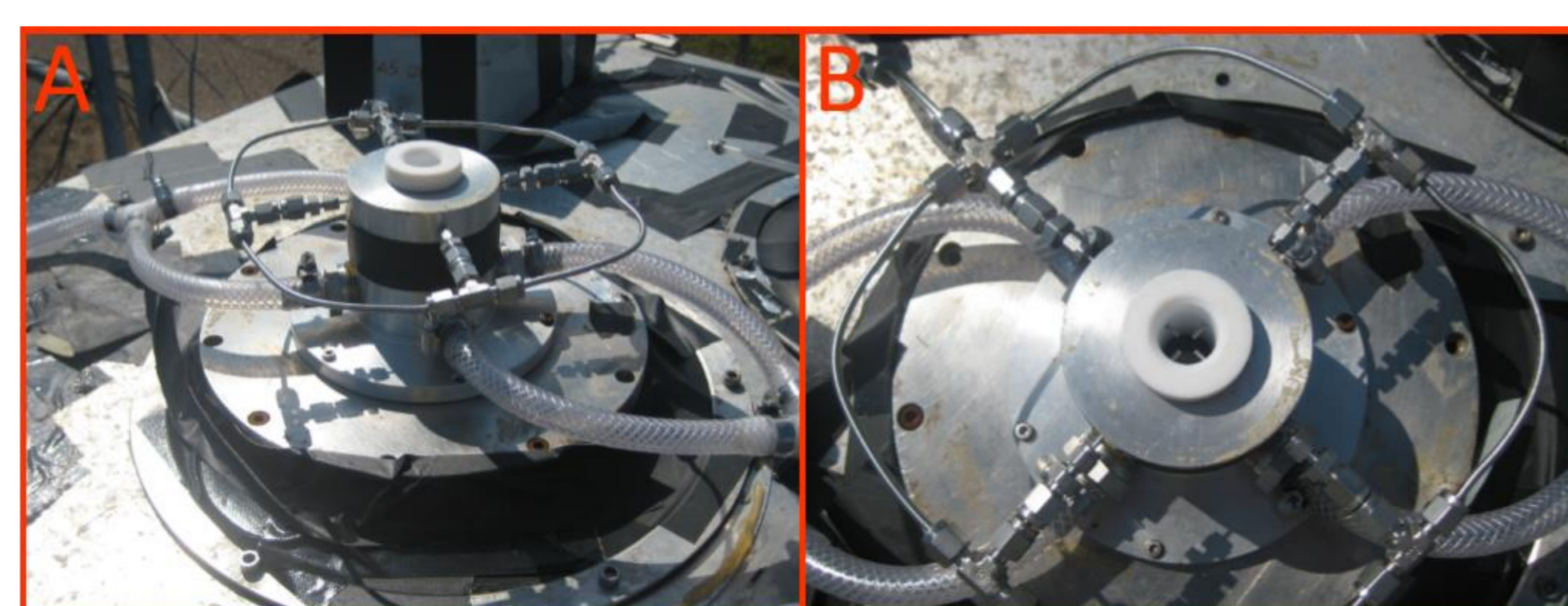
Figure 2 (right). Side (A) and top (B) view photographs of the IPI system, mounted on the HO 2 fluorescence cell. A scroll pump pulls air through four 3/4" holes located just above the base flange of the IPI to provide the sheath flow.
