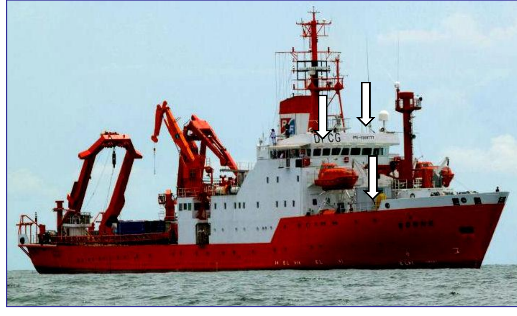
Research Vessel Sonne during SO218 scientific cruise. Arrows mark position of LIF, MAX-DOAS and CE-DOAS IO instruments during cruise. Photo: Johannes Lampel.
