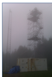
Figure 3 , photo of FAGE instrument at the Schmücke site during a cloud event. Radicals were sampled from the top of the 22 m tower alongside ancillary measurements.
